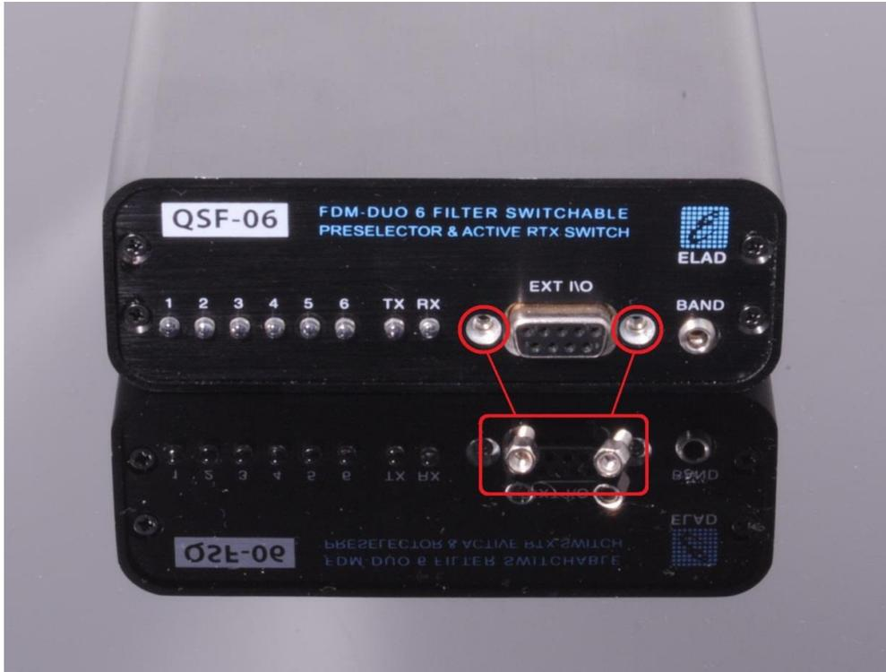
Then, remove the four screws of the rear panel.
