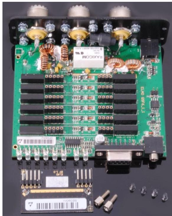
At last, relocate the printed circuit board inside the enclosure and screw in the four screws and the two standoffs.
